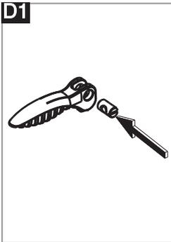
4. Insert the Barrel Nut into the Cam Lock as illustrated in **fig D1**.
